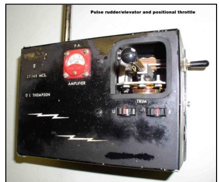
Dan's 1964 Pulse Transmitter with Rudder, Elevator, Throttle (Photo by Dan Thompson)
