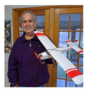
Finally completed my Eaglet 250, after 3 years of building (See picture). It is electric with a dummy 0.020 engine, covered with Ultracote.
