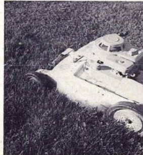
Mower uses an offset front wheel and grass exit. Note attach point.
