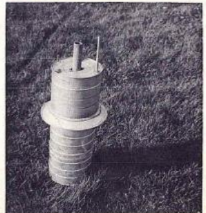
Three cans, a pie plate, a piece of 3/4" pipe, and a length of cable.
