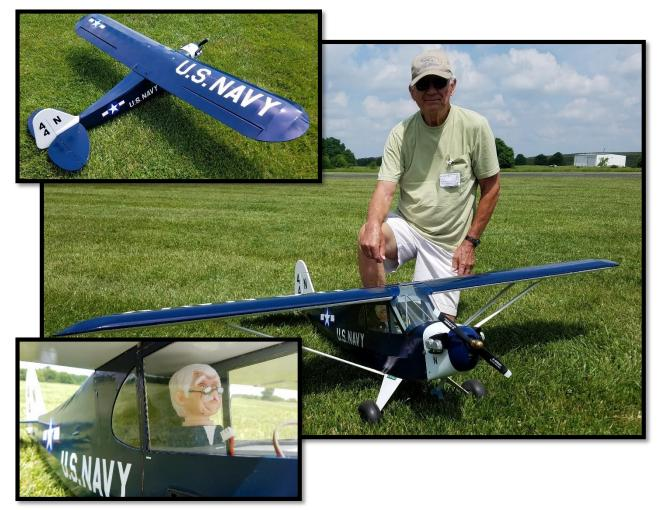
Lee Wright won the Model of the Month with his J-3 at the June Club meeting. The plane was built from a Great Planes kit and is powered by a Maximum .61 engine with a Top Flite incowl muffler. It is covered with Century 21 fabric and the dry weight is 14 lbs. The wing span per plans is 90 inches, but was built as a 83 inch clipped wing. Lee built the J-3 in Florida during the past two winters, and was brought to Lexington this spring. It has not been flown.
