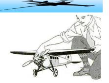
Here is an advertisement for Brown Jr. Motors from the February 1938 issue of Model Airplane News. Mr. Bill Brown, IV is acknowledged to have produced the first practical production gas engine for flying model aircraft (www.craftsmanshipmuseum.com). The cylinder behind the engine is the fuel tank and the cylinder with the wire is the spark plug condenser. Based on inflation, the \$17.00 model would cost \$291.00 today.
