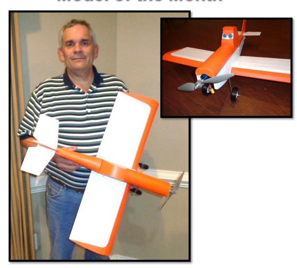
Dave Price won the Model of the Month with his Little Duster plane. Dave scratch built this model from plans downloaded from the Flitetest.com website using sheets of poster foam boards from Dollar Tree store. This 29 inch wing span airplane has a full four channel remote control and is powered by a 2122-1000kv brushless motor with a 3s LiPo battery. Plastic wheels were made on his 3-D printer. An air brush paint job finishes off this nice looking plane.
