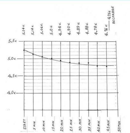
In February 2009, an 800 Miliampere-hour, NiCad Battery pack was installed in the Rearwin Speedster. After a 12 hour charge cycle, a 175 Milliampere 'Load' was placed on the pack continuously and the above voltages plotted.
