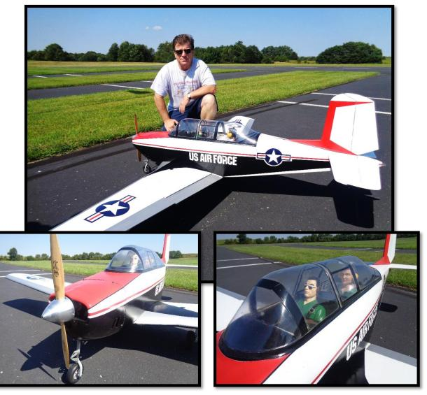
Mickey Breunig won the Model of the Month with his USAF T-34. The 80 inch wing span plane weighs 16 lbs and is powered by a OS91FX 2 stroke glow engine. It was fully equipped with Robart retracts. The military markings on this perfectly built plane were beautifully done.
