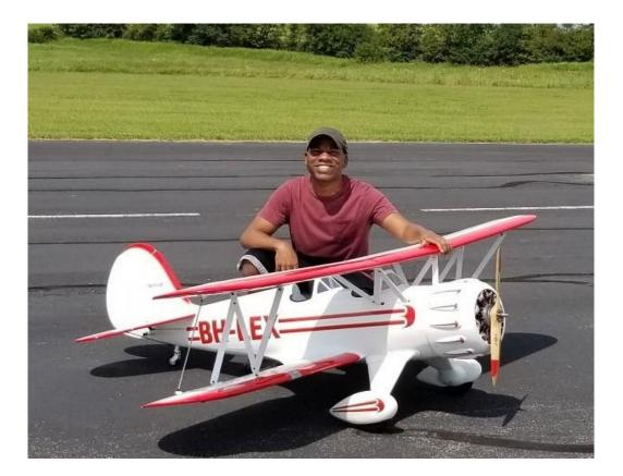
SPECS Phoenix Models WINGSPAN 91" WEIGHT 28 POUNDS MOTOR Zenoah G-62 Futaba Radio Gear
